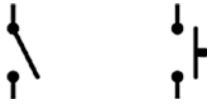
Figure 9-1. Schematic Symbols for an SPST Switch (Left) and an SPST Button (Right)
