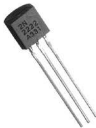
Figure 24-3. A 2N2222A Transistor in a TO-92 Package
