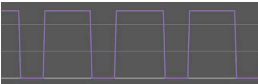
Figure 19-2. A Graph of the Output Voltage in a 555 Oscillator
